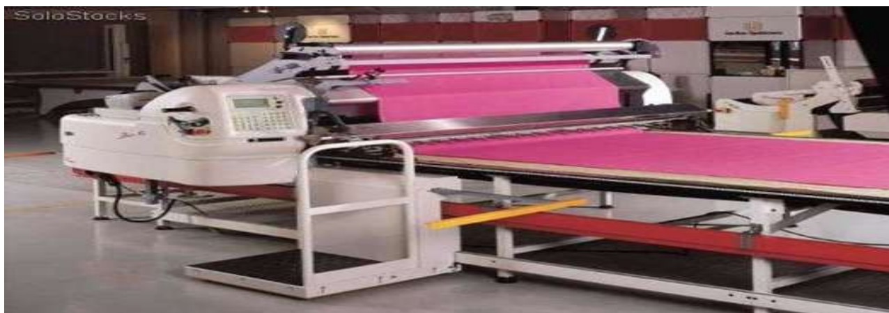
5-rasm. Progress Brio 55G100 gazlamalarni to'shash va bichish mashinasi.
