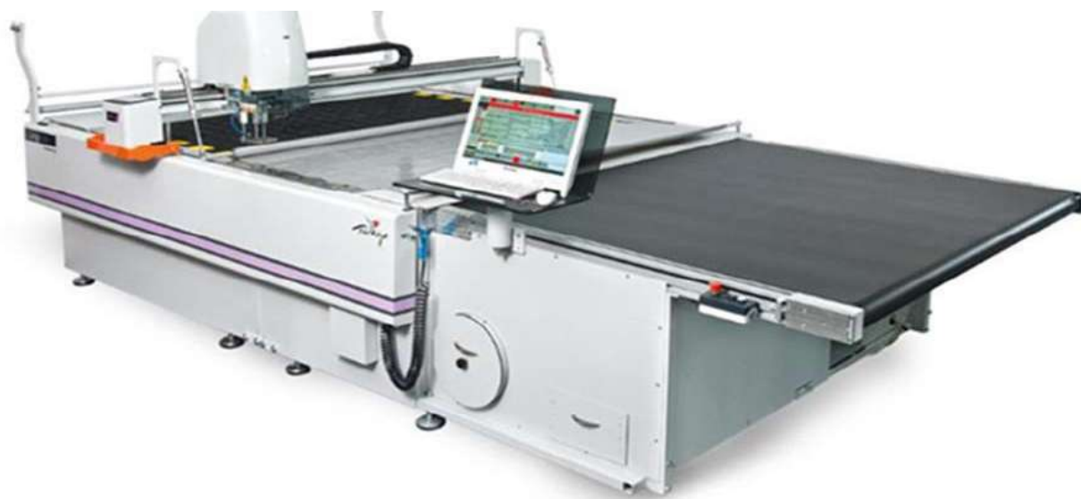
4-rasm. (Investronica Topaz) NT CV070- avtomatik to'shash-bichish mashinasi
